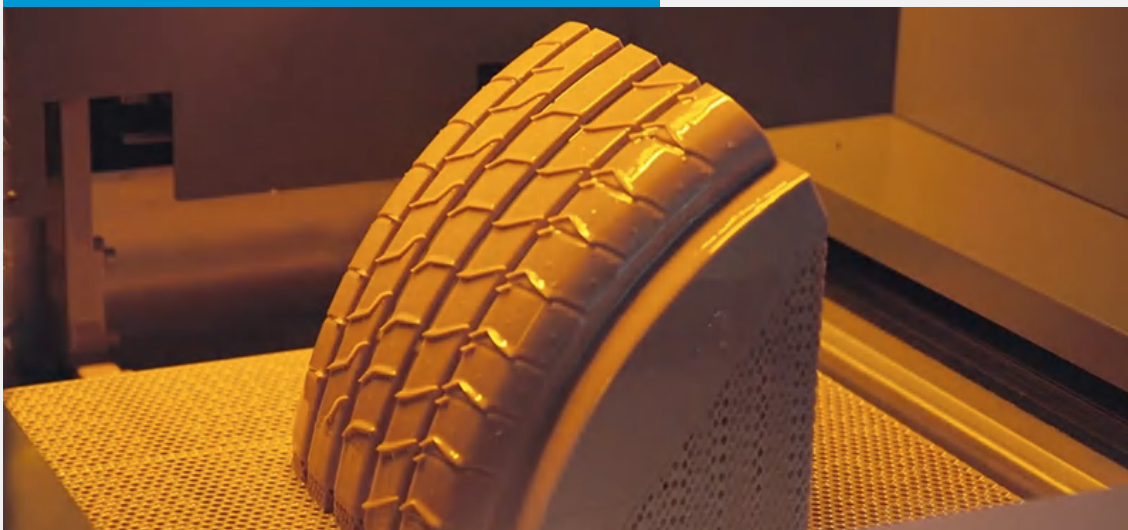
3D Printed Segmented Tire Mold
