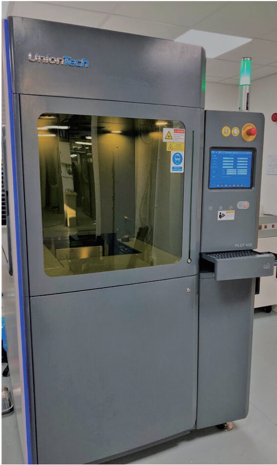
The materials running on this machine are Somos® Waterclear Ultra and Accura Xtreme Grey.
